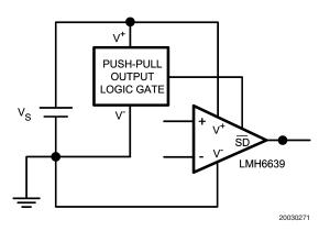
FIGURE 4. Shutdown Interface (Single Supply)
