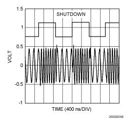
FIGURE 3. Switching between 5 and 10MHz
