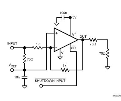
FIGURE 1. Typical Single Supply Schematic
