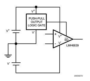
FIGURE 5. Shutdown Interface (Dual Supplies)
