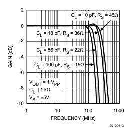
FIGURE 8. Frequency Response vs. Capacitive Load
