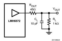
FIGURE 6. Decoupling Capacitive Loads
