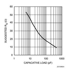
FIGURE 7. Recommended R<sub>OUT</sub> vs. Capacitive Load
