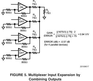
An alternate approach would be to tie the outputs directly together and let all devices share a common back termination resistor in order to alleviate the gain error issue above.
