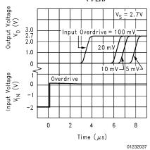
**Typical Performance Characteristics** V<sup>+</sup> = 5V, Single Supply, T<sub>A</sub> = 25°C unless otherwise specified (Continued) **Response Time for Response Time**
