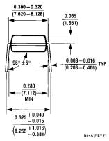
14-Pin Molded Dual-In-Line Package Order Number LMC6574AIN or LMC6574BIN NS Package Number N14A
