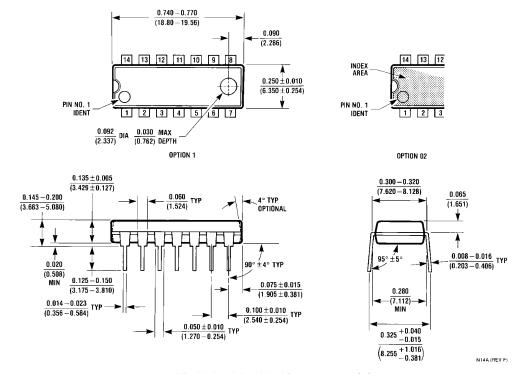
14-Pin Molded Dual-In-Line Package (N)
