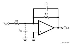
FIGURE 1. Cancelling the Effect of Input Capacitance
