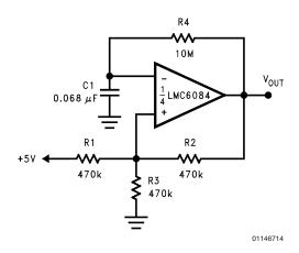
FIGURE 9. 1 Hz Square Wave Oscillator
