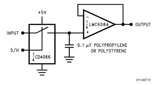
FIGURE 8. Low-Leakage Sample and Hold
