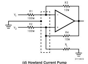
FIGURE 6. Guard Ring Connections
