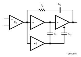
FIGURE 1. LMC6032 Circuit Topology (Each Amplifier)
