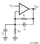
$C_S$  consists of the amplifier's input capacitance plus any stray capacitance from the circuit board and socket.  $C_F$  compensates for the pole caused by  $C_S$  and the feedback resistor.
