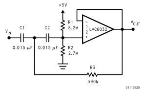
$f_c = 10 \text{ Hz}$ d = 0.895Gain = 1 2 dB passband ripple
