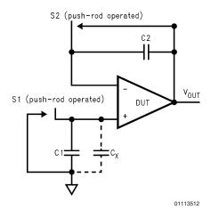
FIGURE 8. Simple Input Bias Current Test Circuit
