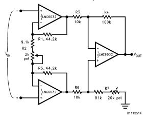
$$\frac{V_{OUT}}{V_{IN}} = \frac{R2 + 2R1}{R2} \times \frac{R4}{R3}$$
