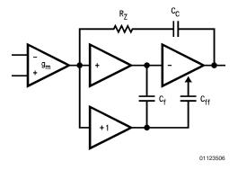
FIGURE 1. LMC6024 Circuit Topology (Each Amplifier)
