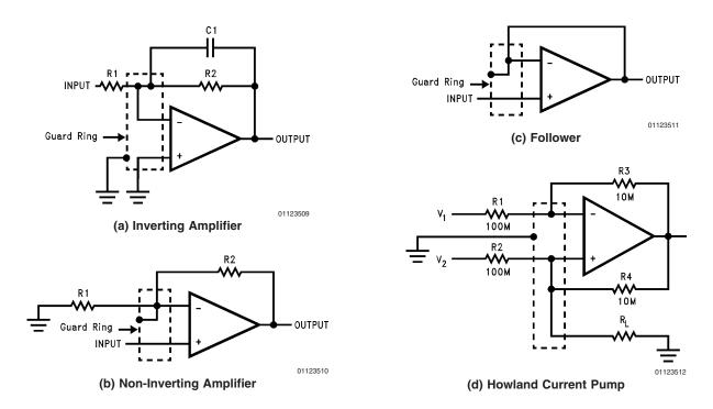
FIGURE 5. Guard Ring Connections
