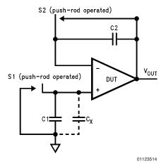
FIGURE 7. Simple Input Bias Current Test Circuit
