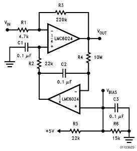
$$\label{eq:Gain} \begin{split} & \text{Gain} = -46.8 \\ & \text{Output offset voltage reduced to the} \\ & \text{level of the input offset voltage of} \\ & \text{the bottom amplifier (typically 1 mV),} \\ & \text{referred to $V_{BIAS}$.} \end{split}$$
