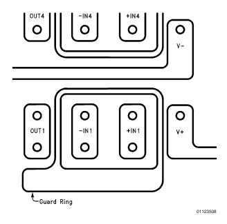
FIGURE 4. Example of Guard Ring in P.C. Board Layout (Using the LMC6024)
