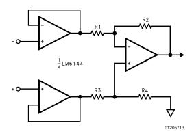
The gain is set by the ratio of R2/R1 and R3 should equal R1 and R4 equal R2. Making R4 slightly smaller than R2 and adding a trim pot equal to twice the difference between R2 and R4 will allow the CMR to be adjusted for optimum.
