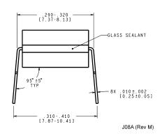
8-Pin Cerdip **Dual-In-Line Package NS Package Number J08A**
