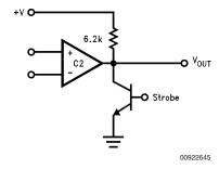
FIGURE 16. Basic Comparator with External Strobe
