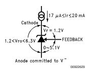
FIGURE 1. Voltage Associated with Reference (current source I, is external)
