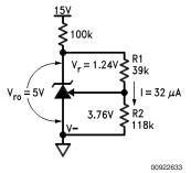
$\begin{aligned} R1 &= Vr/I = 1.24/32 \mu = 39k \\ R2 &= R1 \; \{ (Vro/Vr) - 1 \} = 39k \; \{ (5/1.24) - 1) \} = 118k \end{aligned}$
