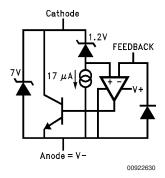
FIGURE 2. Reference Equivalent Circuit
