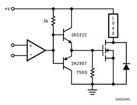
FIGURE 12. High Current, High Voltage Switch
