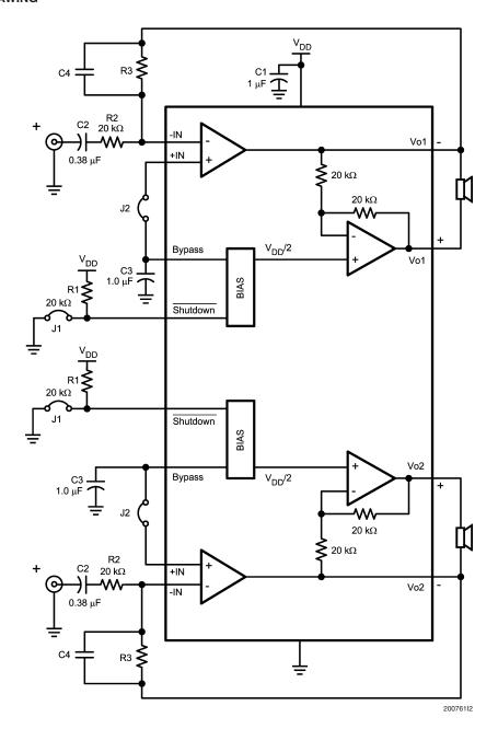
FIGURE 2. Higher Gain Schematic Drawing
