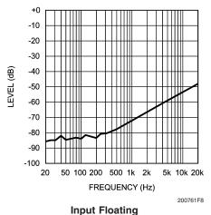
Power Supply Rejection Ratio (PSRR) vs Frequency
