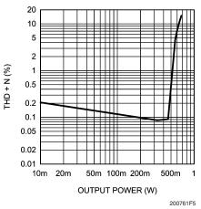
THD+N vs Power Out at  $V_{DD}$  = 2.6V,  $8\Omega R_L$ , 1kHz, per channel
