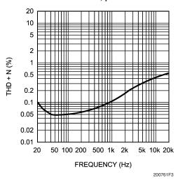
THD+N vs Frequency at  $V_{DD} = 3.3V$ ,  $8\Omega R_L$ , and PWR = 250mW, per channel
