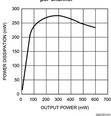
Power Dissipation vs Output Power, 2.6V,  $8\Omega$ , per channel
