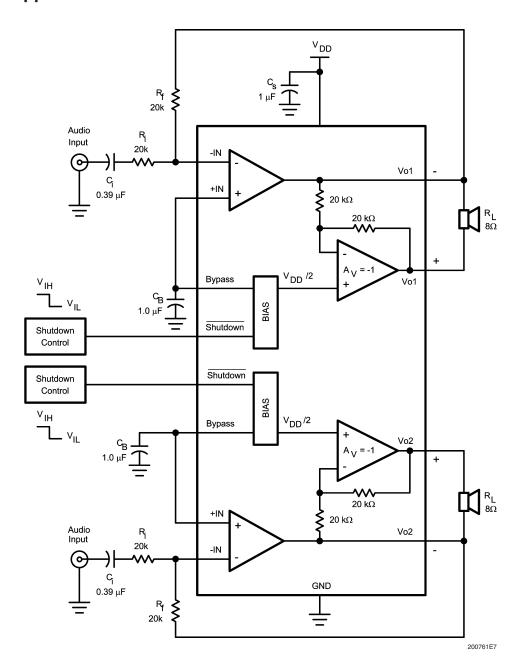
FIGURE 1. Typical Audio Amplifier Application Circuit
