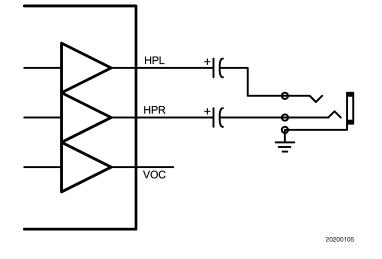
FIGURE 4. Capacitor Coupled Headphone Mode
