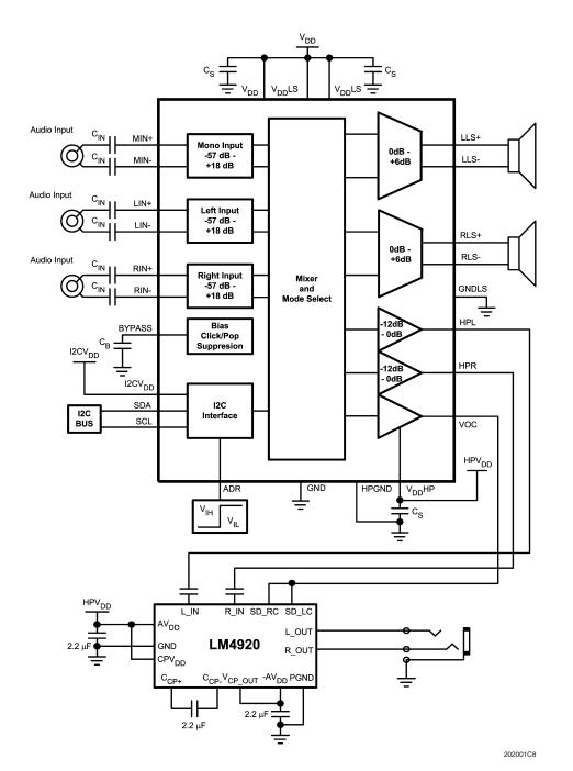
FIGURE 5. Driving an External Headphone Amplifier
