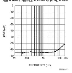
PSRR vs Frequency OCL Headphone Mode, Single-Ended Input Stereo and Mono Inputs Active
