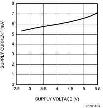
Supply Current vs Supply Voltage Speaker and OCL Headphone Mode, No Load
