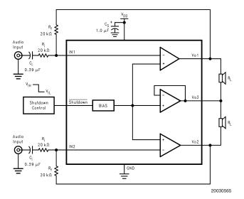
FIGURE 1. Typical Audio Amplifier Application Circuit
