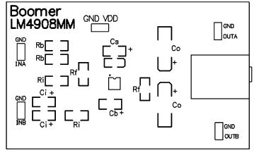
Recommended MSOP Board Layout: Top Overlay
