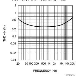
THD+N vs Frequency  $V_{DD}$  = 3.3V, PWR = 25mW,  $R_L$  = 8 $\Omega$
