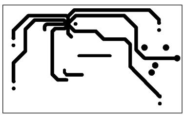
Recommended MSOP Board Layout: Bottom Layer
