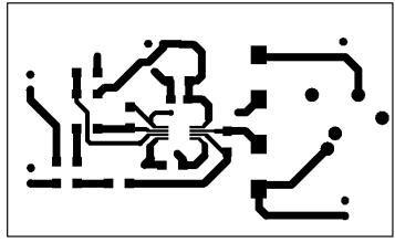
Recommended MSOP Board Layout: Top Layer 20075265
