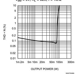
THD+N vs Output Power  $V_{DD}$  = 3.3V,  $R_L$  = 32 $\Omega$ , f = 1kHz
