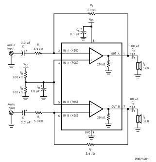
\*Refer to the Application Information Section for information concerning proper selection of the input and output coupling capacitors.
