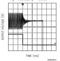
$\begin{aligned} & \text{Fade-In} \\ V_{\text{DD}} &= 5\text{V}, \ R_{\text{L}} = 8\Omega, \ \text{f} = 1\text{kHz} \\ R_{\text{i}} &= 47\text{k}\Omega, \ R_{\text{f}} = 47\text{k}\Omega \end{aligned}$
