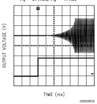
$\begin{aligned} & & Fade\text{-Out} \\ V_{DD} = 5V, \ R_L = 8\Omega, \ f = 1k\text{Hz} \\ R_i = 47k\Omega, \ R_f = 47k\Omega \end{aligned}$
