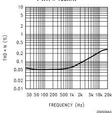
THD+N vs Frequency  $V_{DD}$  = 3V,  $R_L$  =  $8\Omega$  PWR = 150mW
