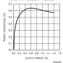
**Power Dissipation vs Output Power**  $V_{DD} = 2.6V$ , f = 1kHz
