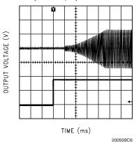
$\begin{aligned} & \text{Fade-In} \\ \textbf{V}_{\text{DD}} &= 5 \text{V}, \ \textbf{R}_{\text{L}} = 8 \Omega, \ \textbf{f} = 1 \text{kHz} \\ \textbf{R}_{\text{i}} &= 9.4 \text{k} \Omega, \ \textbf{R}_{\text{f}} = 47 \text{k} \Omega \end{aligned}$
