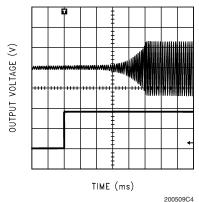
$\begin{aligned} & \text{Fade-In} \\ \textbf{V}_{\text{DD}} &= 5 \text{V}, \ \textbf{R}_{\text{L}} = 8 \Omega, \ \textbf{f} = 1 \text{kHz} \\ \textbf{R}_{\text{i}} &= 10 \text{k} \Omega, \ \textbf{R}_{\text{f}} = 10 \text{k} \Omega \end{aligned}$
