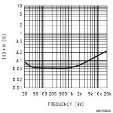
THD+N vs Frequency  $V_{DD}$  = 2.6V,  $R_L$  =  $8\Omega$  PWR = 100mW
