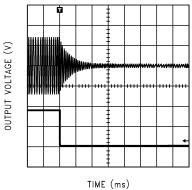
$\label{eq:vdd} \begin{aligned} & \text{Fade-Out} \\ & \text{V}_{\text{DD}} = \text{5V}, \ \text{R}_{\text{L}} = \text{8}\Omega, \ \text{f} = \text{1kHz} \end{aligned}$
