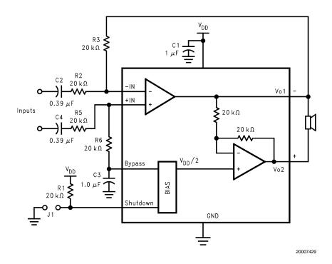
FIGURE 3. Differential Amplifier Configuration for LM4891
