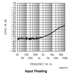
Power Supply Rejection Ratio (PSRR) @ V<sub>DD</sub> = 2.6V
