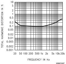
THD+N vs Frequency at  $V_{DD}$  = 2.6V,  $8\Omega$  R<sub>L</sub>, and PWR = 100mW
