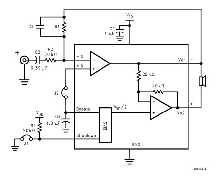
FIGURE 2. Higher Gain Audio Amplifier
