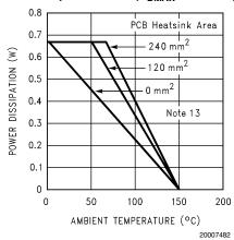
Power Derating - 10 Pin LD Pkg  $P_{DMAX}$  = 670mW, 5V,  $8\Omega$
