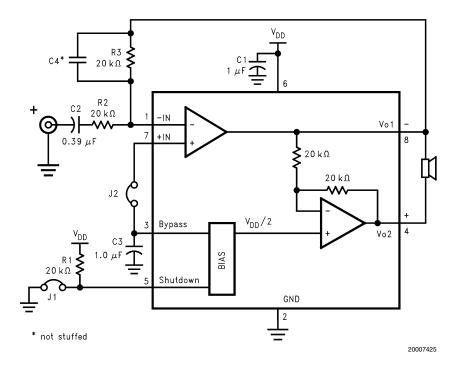
FIGURE 4. Reference Design Board and Layout - micro SMD
