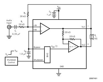
FIGURE 1. Typical Audio Amplifier Application Circuit
