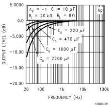
Frequency Response vs Output Capacitor Size
