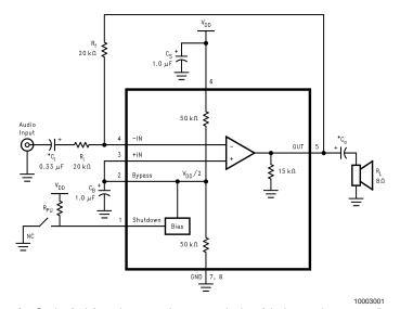
\*Refer to the **Application Information** Section for information concerning proper selection of the input and output coupling capacitors.
