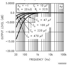
Frequency Response vs Input Capacitor Size
