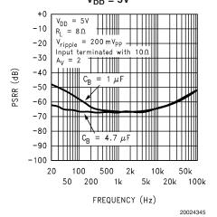
**Power Supply Rejection Ratio**  $V_{DD} = 2.6V$
