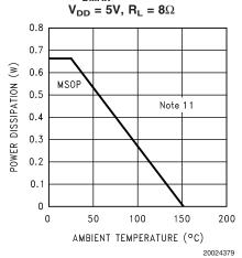
Power Derating - 9 Bump  $\mu$ SMD  $P_{DMAX} = 670mW$   $V_{DD} = 5V, \, R_L = 8\Omega$
