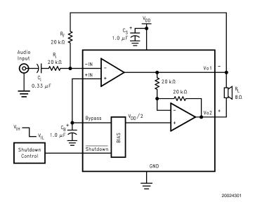
FIGURE 1. Typical Audio Amplifier Application Circuit
