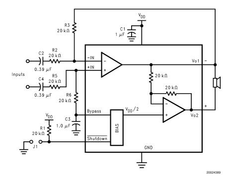
FIGURE 3. DIFFERENTIAL AMPLIFIER CONFIGURATION FOR LM4879
