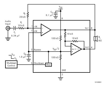
FIGURE 1. Typical Audio Amplifier Application Circuit
