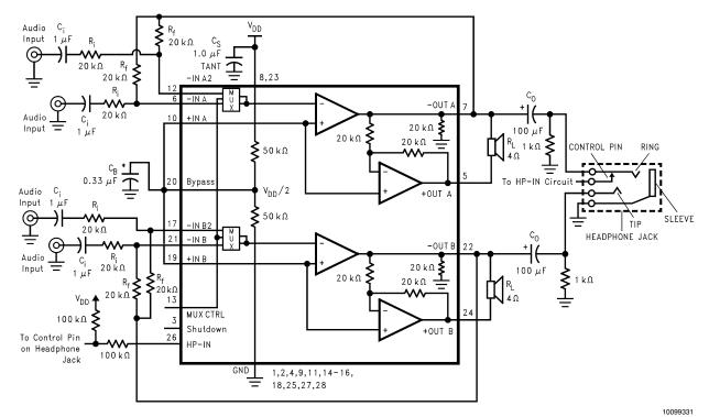
Note: Pin out shown for the 28-pin Exposed-DAP TSSOP package. Refer to the Connection Diagrams for the pin out of the 20-pin Exposed-DAP TSSOP, Exposed-DAP LLP, and micro SMD packages.
