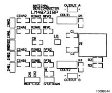
Figure 12. Recommended 20-pin micro SMD PC Board Layout:
