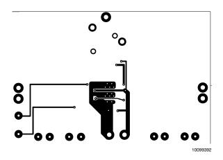
FIGURE 6. Recommended MTE PC Board Layout:
