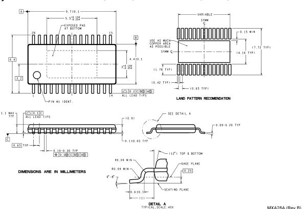
28-Lead MOLDED TSSOP, EXPOSED PAD, 9.7x4.4x0.9mm Order Number LM4873MTE-1 **NS Package Number MXA28A**
