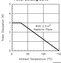
Note 21: This curve shows the LM4873MTE's and the LM4873LQ's thermal dissipation ability at different ambient temperatures given these conditions: 500LFPM + JEDEC board: The part is soldered to a 1S2P 20-lead exposed-DAP TSSOP test board with 500 linear feet per minute of forced-air flow across it. Board information - copper dimensions: 74x74mm, copper coverage: 100% (buried layer) and 12% (top/bottom layers), 16 vias under the exposed-DAP.
