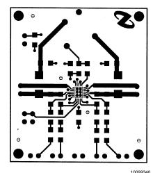
Figure 8. Recommended LQ PC Board Layout: Component-Side Layout
