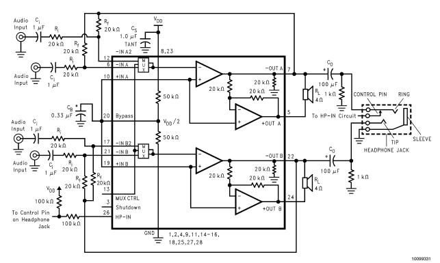
$^{*}$  Refer to the section Selecting Proper External Components, for a detailed discussion of  $C_{B}$  size.
