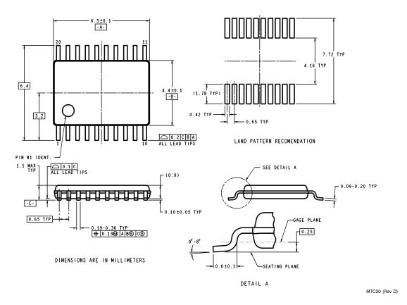
20-Lead MOLDED PKG, TSSOP, JEDEC, 4.4mm BODY WIDTH Order Number LM4873MT NS Package Number MTC20
