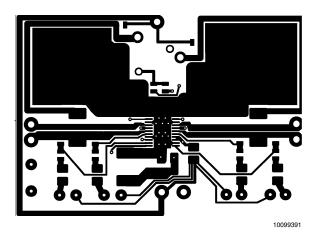
FIGURE 5. Recommended MTE PC Board Layout: Component-Side Layout
