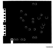
Figure 16. Recommended 20-pin micro SMD PC Board Layout:
