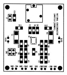
Figure 7. Recommended LQ PC Board Layout: Component-Side Silkscreen
