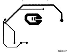
Figure 15. Recommended 20-pin micro SMD PC Board Layout:
