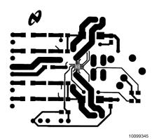
Figure 13. Recommended 20-pin micro SMD PC Board Layout:
