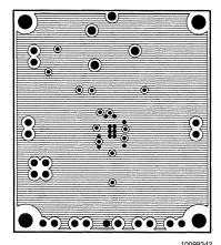
Figure 11. Recommended LQ PC Board Layout:
