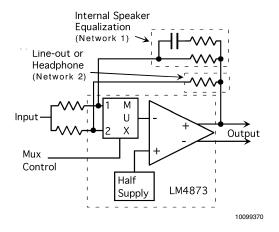
FIGURE 1. Input MUX Example
