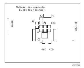
FIGURE 2. Recommended LD PC Board Layout: Component-Side Silkscreen
