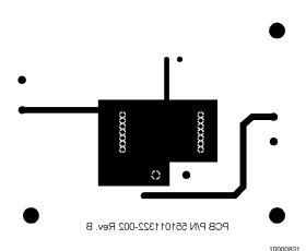
FIGURE 4. Recommended LD PC Board Layout:
