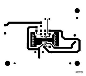
FIGURE 3. Recommended LD PC Board Layout: Component-Side Layout
