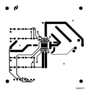
FIGURE 15. Recommended MTE PC Board Layout: Component-Side Layout
