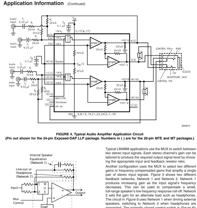
FIGURE 5. Input MUX Example
