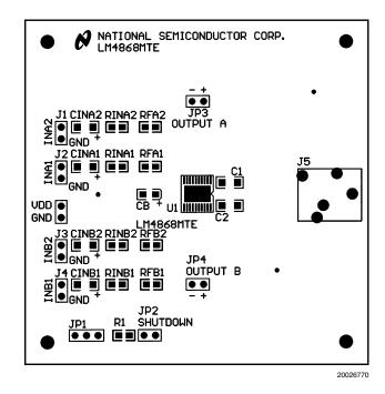
FIGURE 14. Recommended MTE PC Board Layout: Component-Side Silkscreen
