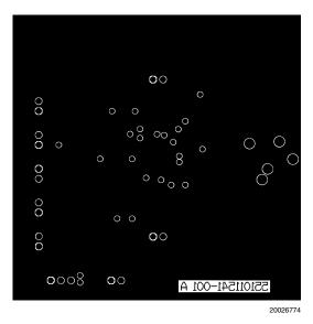
FIGURE 18. Recommended MTE PC Board Layout: Bottom-Side Layout
