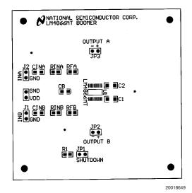
FIGURE 12. Recommended MT PC board layout: component-side silkscreen
