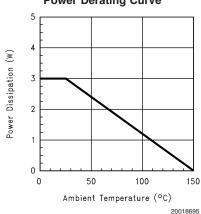
**Note 17:** This curve shows the LM4866LQ's thermal dissipation ability at different ambient temperatures given this condition: The LLP package's DAP is soldered to a 2.5in<sup>2</sup>, 1oz. copper plane.
