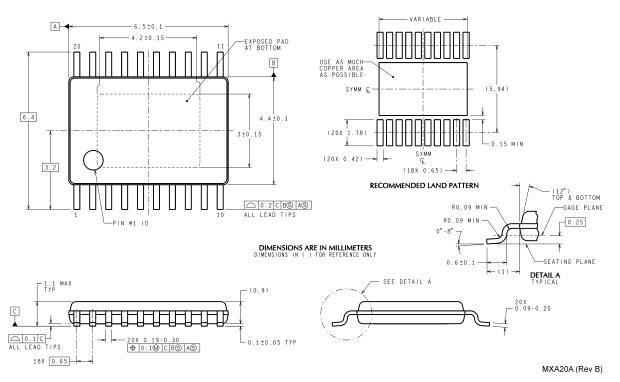
20-Lead Molded TSSOP, Exposed Pad, 6.5x4.4x0.9mm Order Number LM4866MTE NS Package Number MXA20A
