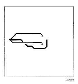
FIGURE 9. Recommended MTE board layout: upper inner-layer layout
