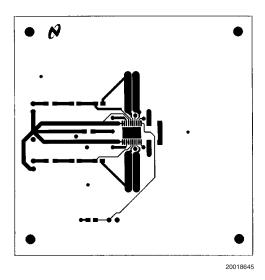
FIGURE 8. Recommended MTE PC board layout: component-side layout
