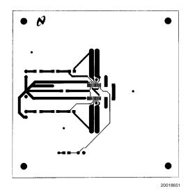
FIGURE 13. Recommended MT board layout: component-side layout
