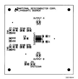
FIGURE 7. Recommended MTE board layout: component-side silkscreen
