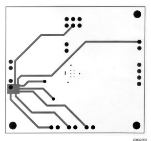
FIGURE 10. Recommended LD PC Board Layout: Inner Layer 2
