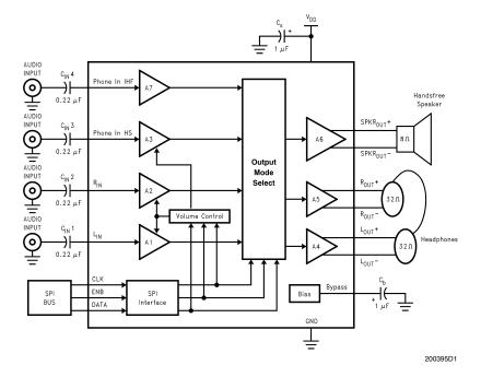
FIGURE 1. Typical Audio Amplifier Application Circuit
