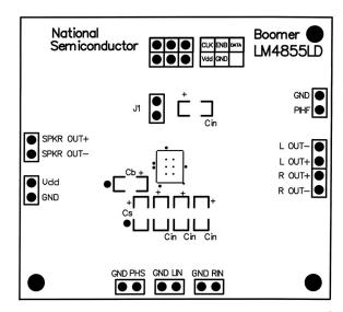
FIGURE 7. Recommended LD PC Board Layout:
