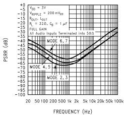
**Power Supply Rejection Ratio**
