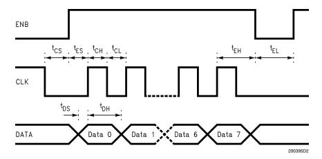
FIGURE 2. SPI Timing Diagram
