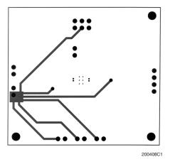
FIGURE 10. Recommended LQ PC Board Layout: Innner Layer 2
