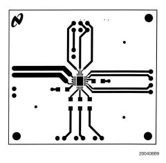
FIGURE 8. Recommended LQ PC Board Layout: Top Layer
