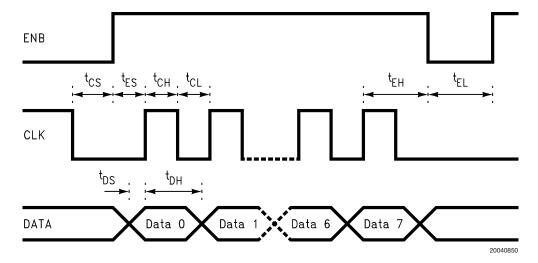
FIGURE 2. SPI Timing Diagram
