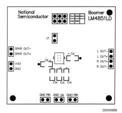
FIGURE 7. Recommended LQ PC Board Layout: Top Silkscreen Layer
