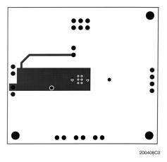
FIGURE 9. Recommended LQ PC Board Layout: Innner Layer 1
