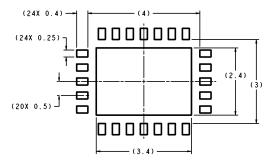
DIMENSIONS ARE IN MILLIMETERS RECOMMENDED LAND PATTERN 1:1 RATION WITH PKG SOLDER PADS
