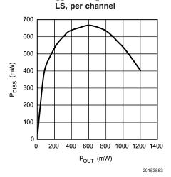
LM4844TL Power Dissipation vs Output Power  ${\rm V_{DD}=3V,\,R_L=8\Omega}$  LS, per channel
