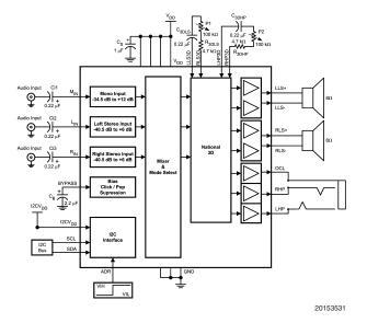
FIGURE 1. Audio Sub-system Block Diagram
