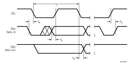
FIGURE 2. I<sup>2</sup>C Timing Diagram
