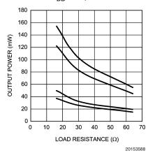
LM4844TL Output Power vs Supply Voltage, HP  $R_L = 32\Omega$ ; Top- 10%THD+N, Bot- 1%THD+N
