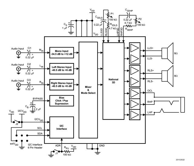
FIGURE 4. Reference Design Board Schematic
