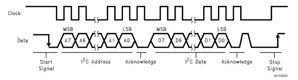
FIGURE 3. I<sup>2</sup>C Bus Format
