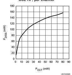
LM4844TL Power Dissipation vs Output Power  $\label{eq:VDD} \textbf{V}_{\text{DD}} = \textbf{3V}, \ \textbf{R}_{\text{L}} = \textbf{32}\Omega$  OCL HP, per channel
