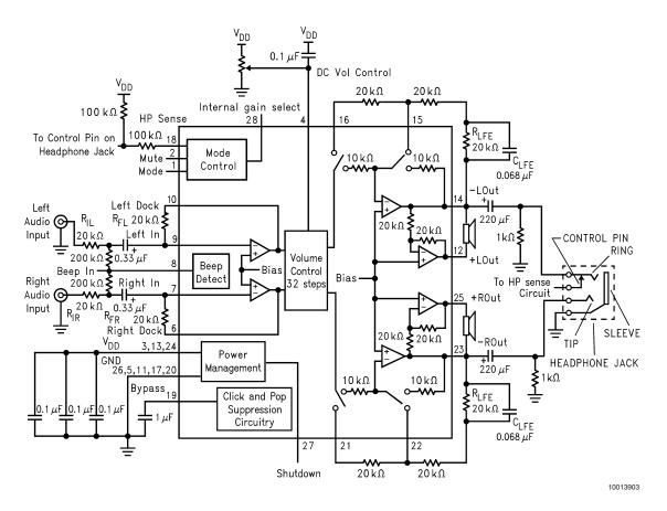
FIGURE 2. Typical Application Circuit
