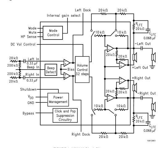
FIGURE 1. LM4835 Block Diagram
