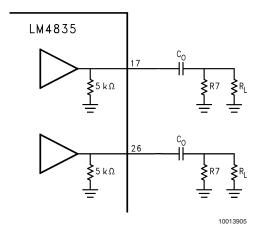
FIGURE 3. Resistor for Varying Output Loads
