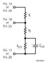
At low, frequencies  $C_{\mathsf{LFE}}$  is a virtual open circuit and at high frequencies, its nearly zero ohm impedance shorts  $R_{\mathsf{LFE}}$ . The result is increased bridge-amplifier gain at low frequencies. The combination of  $R_{\mathsf{LFE}}$  and  $C_{\mathsf{LFE}}$  form with a -3dB corner frequency at
