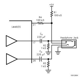
FIGURE 4. Headphone Sensing Circuit
