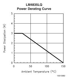
Note 19: These curves show the thermal dissipation ability of the LM4835MTE at different ambient temperatures given these conditions: 500LFPM + 2in<sup>2</sup>: The part is soldered to a 2in<sup>2</sup>, 1 oz. copper plane with 500 linear feet per minute of forced-air flow across it.
