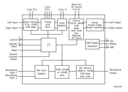
FIGURE 1. LM4832 Block Diagram
