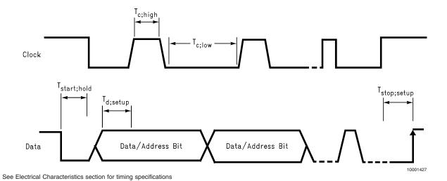
FIGURE 4. I<sup>2</sup>C Timing Diagram
