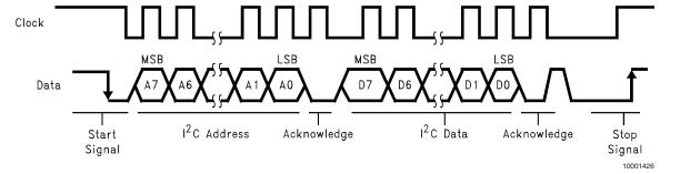
FIGURE 3. I<sup>2</sup>C Bus Format
