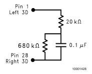
FIGURE 5. 3D Effect Components
