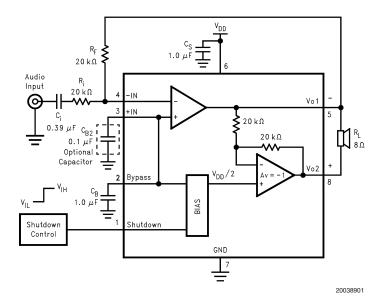
FIGURE 1. Typical Audio Amplifier Application Circuit
