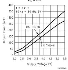
Output Power vs Supply Voltage  $R_L = 16\Omega$
