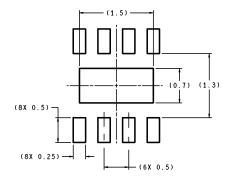
DIMENSIONS ARE IN MILLIMETERS
