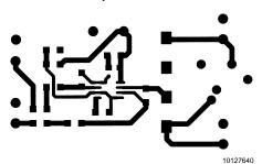
Recommended SOP PC Board Layout: Top Layer
