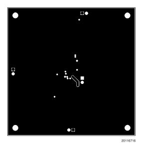
FIGURE 8. Upper Internal GND Layer
