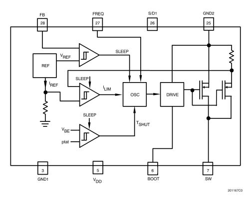
FIGURE 2. Functional Diagram of the LM4804's Regulator
