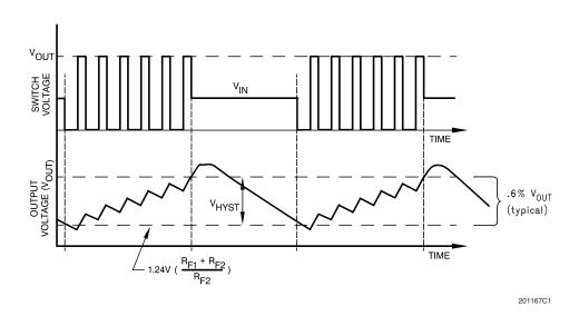
FIGURE 3. Typical Step-Up Regulator Waveforms
