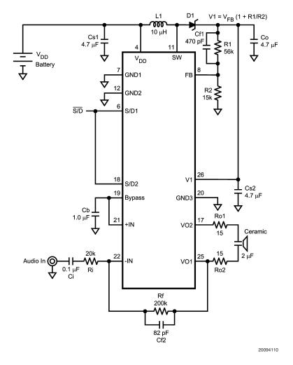
FIGURE 1. Typical Audio Amplifier Application Circuit
