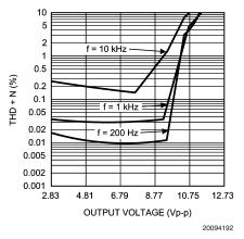
THD+N vs Output Voltage  $V_{DD}$  = 3V,  $Z_L$  = 2 $\mu$ F + 30 $\Omega$ ,  $V_1$  = 5.8V
