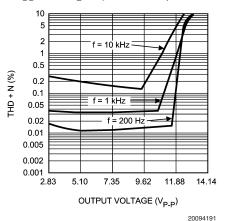
THD+N vs Frequency  $\label{eq:VDD} \text{V}_{\text{DD}} = 4.2 \text{V}, \ \text{Z}_{\text{L}} = 2 \mu \text{F} + 30 \Omega, \ \text{V}_{\text{OUT}} = 10 \text{V}_{\text{P-P}}$
