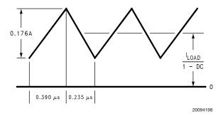
FIGURE 2. 10µH Inductor Current 5V - 12V Boost (LM4802B)
