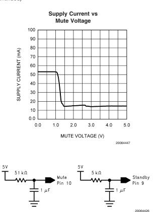
FIGURE 2. Mute and Standby Pin Lowpass Filters
