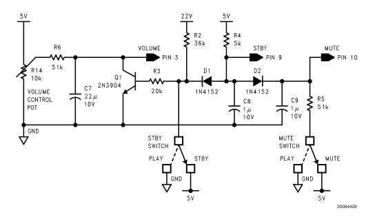
FIGURE 5. Turn-On/Off External Circuitry
