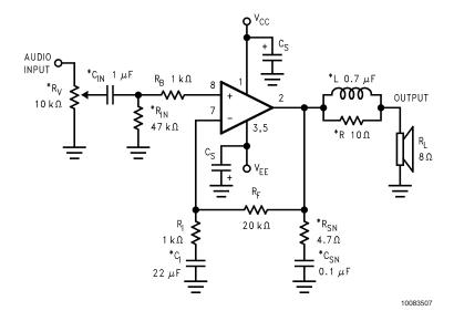
FIGURE 4. Auxillary Amplifier Application Circuit
