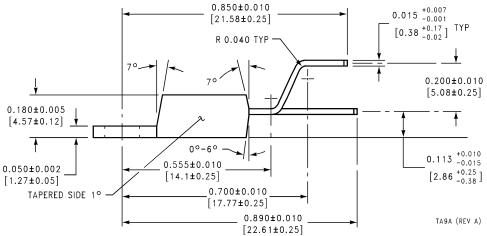
For Staggered Lead Non-Isolated Package Only a 9-Pin Package Order Number LM4701T NS Package Number TA9A
