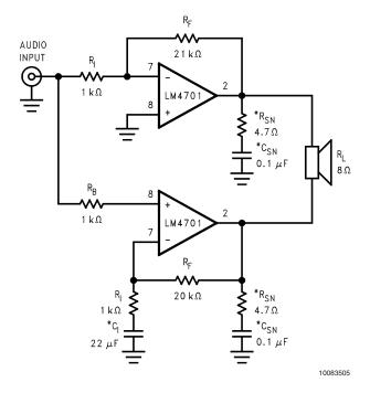
FIGURE 2. Bridged Amplifier Application Circuit
