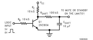
FIGURE 5. Level Shift Circuit
