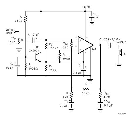
FIGURE 3. Single Supply Amplifier Application Circuit
