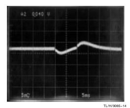
per watt, within the first 10 ms after a step of power is applied. The LM133's specification is 0.01%/W, max.
