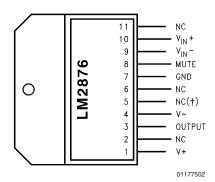
$^{\dagger}\text{Connect Pin 5 to V}^{+}$  for Compatibility with LM3886.
