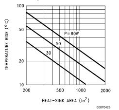
The design of heat sink is beyond the scope of this work. Convection-cooled heat sinks are available commercially, and their manufacturers should be consulted for ratings. The preceding figure is a rough guide for temperature rise as a function of fin area (both sides) available for convection cooling.
