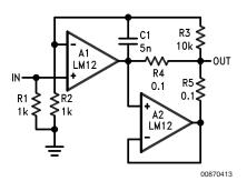
This connection allows increased output capability without requiring a separate control amplifier. The output buffer,  $A_2$ , provides load current through  $R_5$  equal to that supplied by the main amplifier,  $A_1$ , through  $R_4$ . Again, more output buffers can be added.
