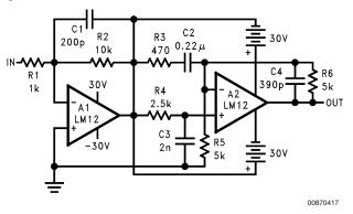
This circuit shows how two amplifiers can be cascaded to double output swing. The advantage over the bridge is that the output can be increased with any number of stages, although separate supplies are required for each.
