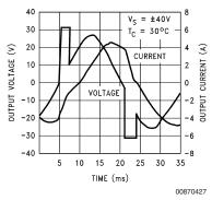
Should the power ratings of the LM12 be exceeded, dynamic safe-area protection is activated. Waveforms with this power limiting are shown for the LM12 driving ±26V at 30 Hz into  $3\Omega$  in series with 24 mH ( $\theta$  = 45°). With an inductive load, the output clamps to the supplies in power limit, as above. With resistive loads, the output voltage drops in limit. Behavior with more complex RCL loads is between these extremes.
