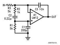
Extending input compensation to the integrator connection is shown here. Both the follower and this integrator will handle 1  $\mu$ F capacitive loading without LR output isolation.
