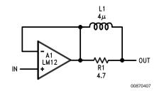
Large capacitive loads (including series-resonant) can be accommodated by isolating the feedback amplifier from the load as shown above. The inductor gives low output impedance at lower frequencies while providing an isolating im-
