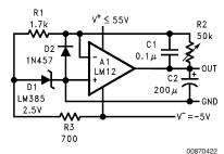
An op amp can be used as a positive or negative regulator. Unlike most regulators, it can sink current to absorb energy dumped back into the output. This positive regulator has a 0-50V output range.
