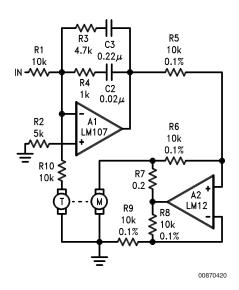
This motor/tachometer servo gives an output speed proportional to input voltage. A low-level op amp is used for frequency shaping while the power op amp provides current drive to the motor. Current drive eliminates loop phase shift due to motor inductance and makes high-performance servos easier to stabilize.
