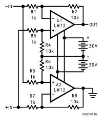
One limitation of the standard bridge connection is that the load cannot be returned to ground. This can be circumvented by operating the bridge with floating supplies, as shown above. For single-ended drive, either input can be grounded.
