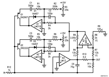
Note: Supply voltages for the LM318s are ±15V
