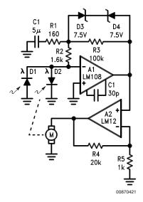
This position servo uses an op amp to develop the rate signal electrically instead of using a tachometer. In highperformance servos, rate signals must be developed with large error signals well beyond saturation of the motor drive. Using a separate op amp with a feedback clamp allows the rate signal to be developed properly with position errors more than an order of magnitude beyond the loop-saturation level as long as the photodiode sensors are positioned with this in mind.
