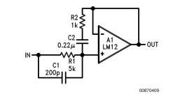
An example of a voltage follower with input compensation is shown here. The  $R_2C_2$  combination across the input works with  $R_1$  to reduce feedback at high frequencies without greatly affecting response below 100 kHz. A lead capacitor,  $C_1$ , improves phase margin at the unity-gain crossover fre-
