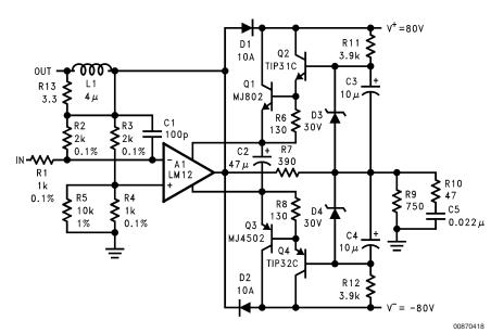
Discrete transistors can be used to increase output drive to  $\pm$ 70V at  $\pm$ 10A as shown above. With proper thermal design,
