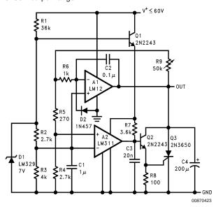
Dual supplies are not required to use an op amp as a voltage regulator if zero output is not required. This 4V to 50V regulator operates from a single supply. Should the op amp not be able to absorb enough energy to control an overvoltage condition, a SCR will crowbar the output.
