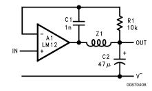
The LM12 can be made stable for all loads with a large capacitor on the output, as shown above. This compensation gives the lowest possible closed-loop output impedance at high frequencies and the best load-transient response. It is appropriate for such applications as voltage regulators.
