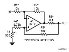
This circuit provides an output current proportional to the input voltage. Current drive is sometimes preferred for servo motors because it aids in stabilizing the servo loop by reducing phase lag caused by motor inductance. In applications requiring high output resistance, such as operational power supplies running in the current mode, matching of the feedback resistors to 0.01% is required. Alternately, an adjustable resistor can be used for trimming.
