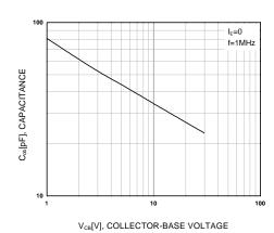
Figure 5. Collector Output Capacitance
