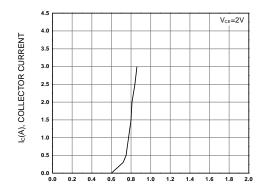
Figure 4. Base-Emitter On Voltage
