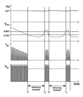
Figure 18. Burst-Mode Operation
