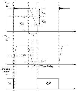
Figure 15. Valley Switching Waveforms
