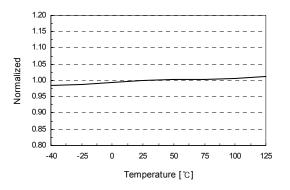
Figure 6. Start Threshold Voltage (V<sub>START</sub>) vs. T<sub>A</sub>
