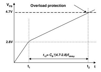
Figure 17. Overload Protection
