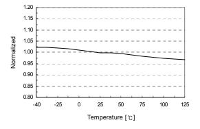
Figure 8. Shutdown Feedback Voltage ( $V_{SD}$ ) vs.  $T_A$
