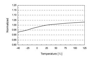
Figure 11. Shutdown Delay Current (I<sub>DELAY</sub>) vs. T<sub>A</sub>
