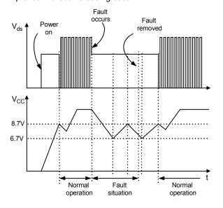
Figure 16. Auto Restart Protection Waveforms
