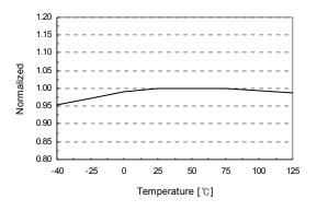
Figure 4. Operating Frequency (fosc) vs. T<sub>A</sub>
