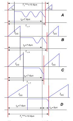
Figure 19. Advanced VS Operation
