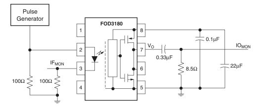
Figure 15. Test Schematic
