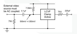
Figure 19. Biased SCART with AC-Coupled Outputs
