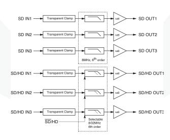
Figure 1. Block Diagram
