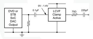
Figure 18. AC-Coupled Inputs, AC-Coupled Outputs
