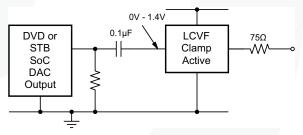
Figure 14. AC-Coupled Inputs, DC-Coupled Outputs
