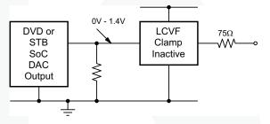
Figure 13. DC-Coupled Inputs and Outputs
