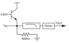
Figure 12. Input Clamp Circuit
