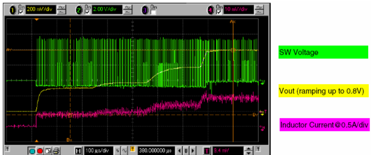
Figure 4: Start-Up Waveform at Full Load V_{in} = 5.5V
