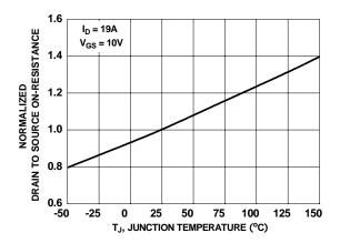
Figure 3. Normalized On-Resistance vs Junction Temperature
