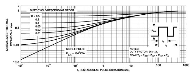
Figure 11. Transient Thermal Response Curve
