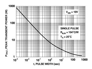
Figure 10. Single Pulse Maximum Power Dissipation
