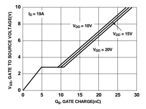
Figure 7. Gate Charge Characteristics
