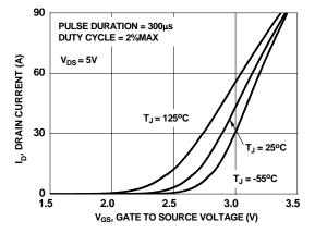
Figure 5. Transfer Characteristics
