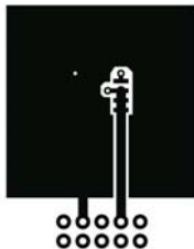
a) 50^\circ\text{C/W} when mounted on a 1\text{in}^2 pad of 2 oz copper.
