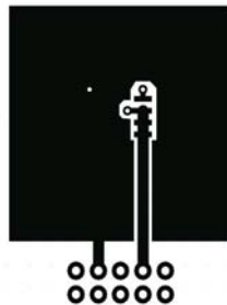
a) 50^\circ\text{C}/\text{W} when mounted on a 1\text{in}^2 pad of 2 oz copper.
