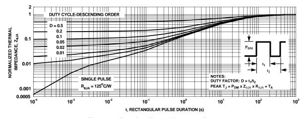
Figure 13. Transient Thermal Response Curve
