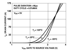
Figure 5. Transfer Characteristics
