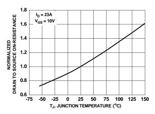
Figure 3. Normalized On-Resistance vs Junction Temperature
