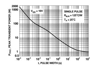
Figure 12. Single Pulse Maximum Power Dissipation
