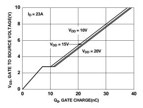
Figure 7. Gate Charge Characteristics
