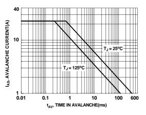
Figure 9. Unclamped Inductive Switching Capability
