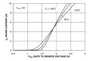
Figure 5. Transfer Characteristics.
