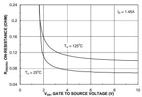
Figure 4. On-Resistance Variation with Gate-to-Source Voltage.
