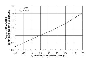
Figure 3. On-Resistance Variation with Temperature.
