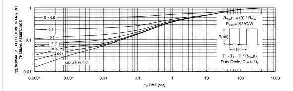
Figure 11. Transient Thermal Response Curve.
