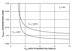
Figure 4. On-Resistance Variation with Gate-to-Source Voltage
