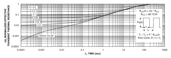
Figure 11. Transient Thermal Response Curve
