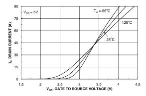
Figure 5. Transfer Characteristics
