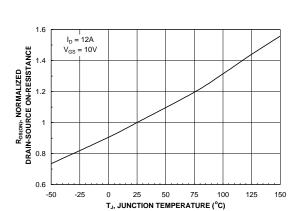
Figure 3. On-Resistance Variation withTemperature
