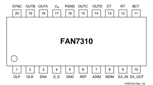
Figure 3. Pin Configuration (Top View)
