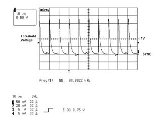
Figure 9. SYNC Waveform
