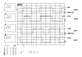
Figure 10. Phase-Shift Control Waveforms
