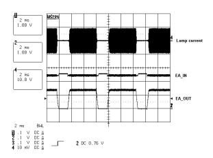
Figure 7. Burst Dimming
