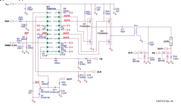
Figure 1. Application Circuit for CCFL
