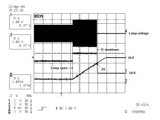
Figure 8. OLR Voltage During Striking Mode
