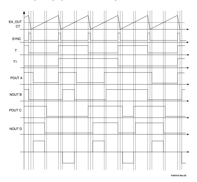
Figure 10. Phase-Shift Control Waveforms
