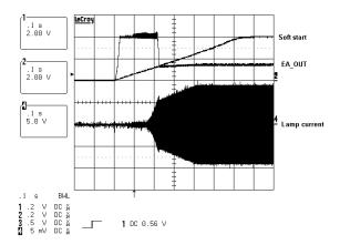
Figure 4. Soft-Start During Initial Operation
