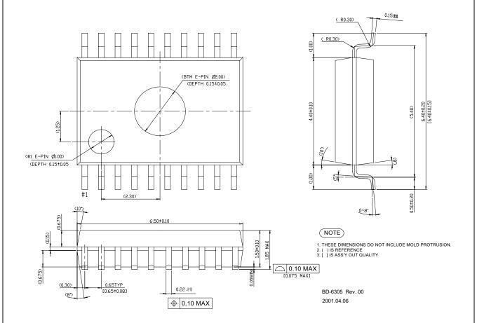
Figure 12. 20-Lead Shrink Small Outline Package (SSOP)
