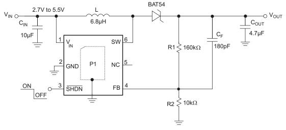
Figure 3. Test Circuit
