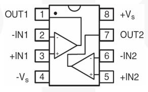
Figure 5. FAN4274 MSOP
