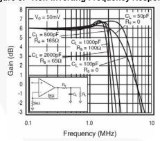
Figure 10. Frequency Response vs. C<sub>L</sub>
