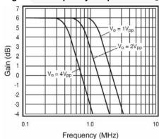
Figure 12. Large Signal Frequency Response (+5V)
