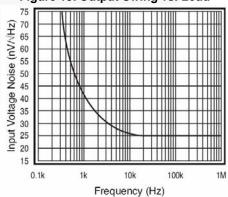
Figure 21. Input Voltage Noise
