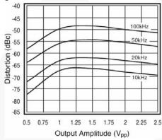
Figure 16. 3rd Harmonic Distortion vs. Vo
