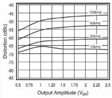
Figure 15. 2nd Harmonic Distortion vs. Vo
