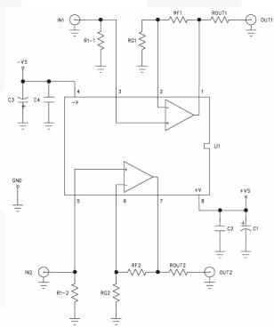
Figure 27. FAN4274 Evaluation Board Schematic (KEB010)
