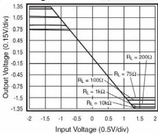
Figure 19. Output Swing vs. Load
