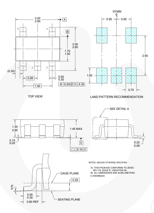
Figure 32. 5-Lead SOT-23 Package
