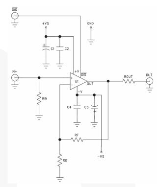
Figure 26. FAN4174 Evaluation Board Schematic (KEV002/KEB011)
