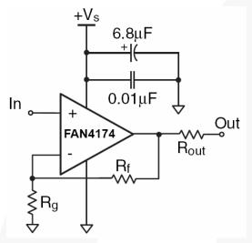
Figure 22. Typical Non-inverting Configuration
