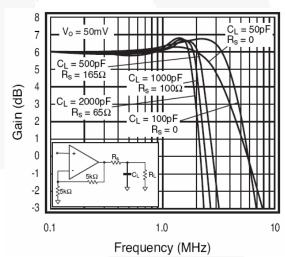
Figure 1. Frequency vs.Gain
