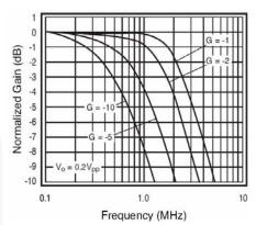
Figure 7. Inverting Frequency Response (+5V)
