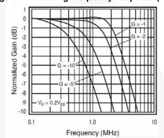
Figure 9. Inverting Frequency Response
