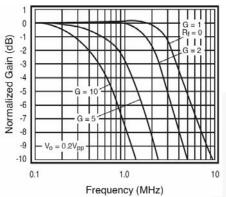
Figure 6. Non-Inverting Frequency Response (+5)
