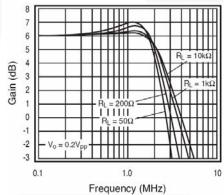
Figure 11. Frequency Response vs. RL
