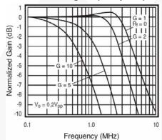
Figure 8. Non-Inverting Frequency Response
