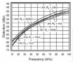
Figure 14. 2nd and 3rd Harmonic Distortion
